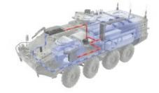
Air heater Water heater Air-conditioning system
