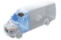
Evaporator integrated into the roof
