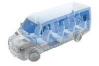
Evaporator vertical on the side at the rear
