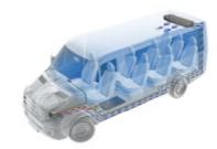
Evaporator under the roof
