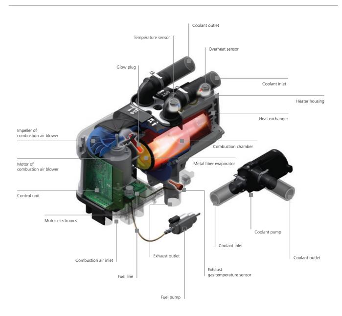
The water heater is incorporated into the vehicle's engine coolant circuit. In this circuit, it flows first through the heat exchanger of the heating system and then through the vehicle's engine.
