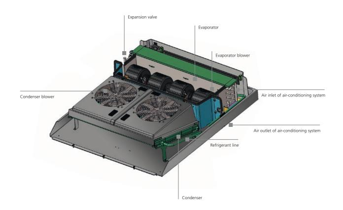
In the closed circuit of the air-conditioning system, a special refrigerant absorbs the heat from the interior of the vehicle and releases it again to the environment at some other point.
