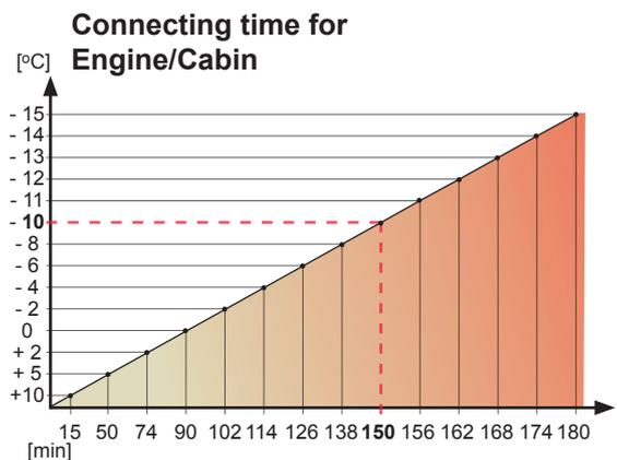
Example: The system will be turned on 150 minutes before pickup time at -10°C (180 minuts at -15°C).
