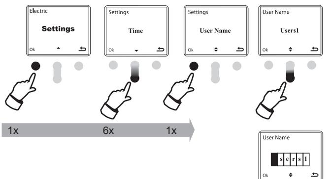
**!** You can switch user under the menu **Users**. To get there press 1x **Menu** , 1x **Arrow down** and 1x **Ok**. Switch user by using **Arrow up/down** and press **Ok** to confirm.
