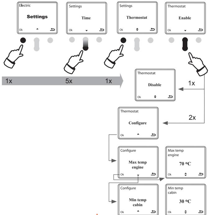
**!** If you are using the temp. sensor as a interior thermostat, a temp. sensor in the VU unit will control the **Aut** program for the engine heater.
