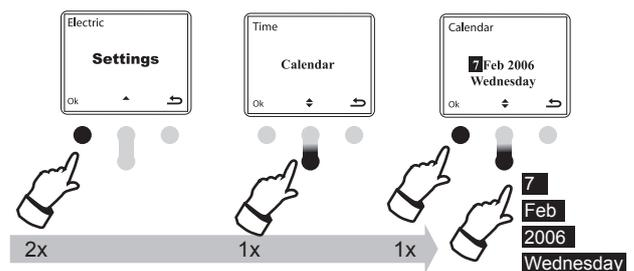
If you press the right key according to point 4, the setting process is interrupted.
