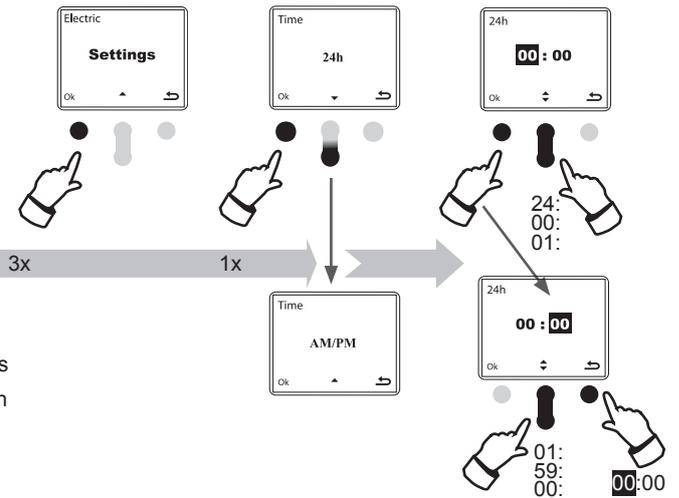
If you press the right key according to point 4, the setting process is interrupted.
