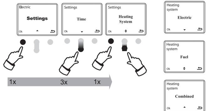
Select **Ok** when the display shows **Fuel** or **Combined** and return twice using **↶**.
