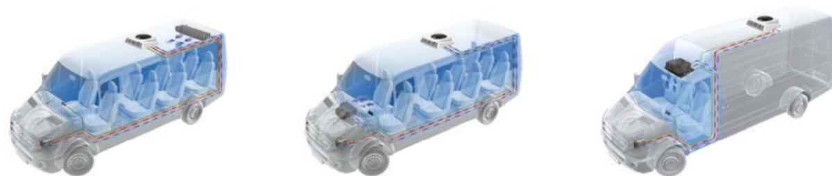
Evaporator under the roof
