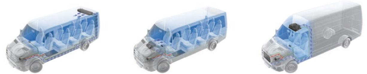
Evaporator under the roof
